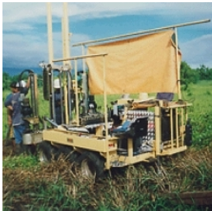
Field CBR test being performed for existing pavement evaluation NAIA IPT3 airport project
