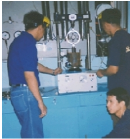
Trial tests on Cement Treated Base (CTB) being performed in controlled strain equipment.
